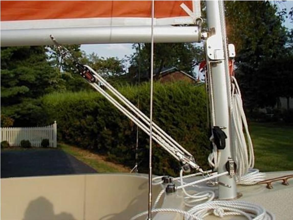
These pictures of the boom vang were taken after the change to Harken blocks, but before the removal of the mast bails and the addition of the horn cleats. the horns will go right in the middle of where the bail will come out.
