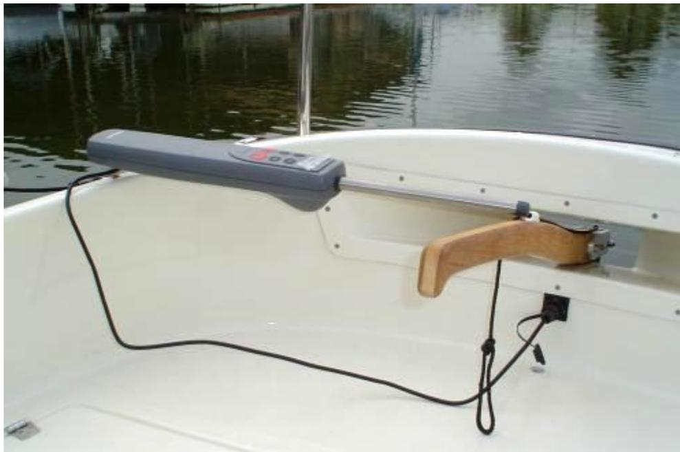
Got in a nice sail after work today. Here are a few pictures of my third sail with the ST1000 tiller pilot. The wind was roughly 10 mph, occasionally up to about 12 or 13, based on the few white caps I saw. I'm still tickled by the SunCat's EASY performance. This picture shows the tiller pilot only a few inches away from the end of its travel. The centerboard was all the way down. I was able to make the tiller pilot "bottom out" at the end of its travel with the centerboard all the way down.
