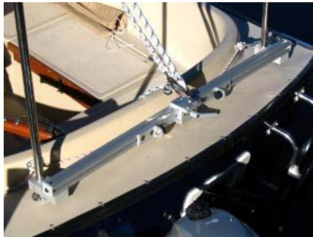
Here is the close up of the traveler mounting hardware. The hardware clamps to the boom cradle upright just below the strut for added strength.
