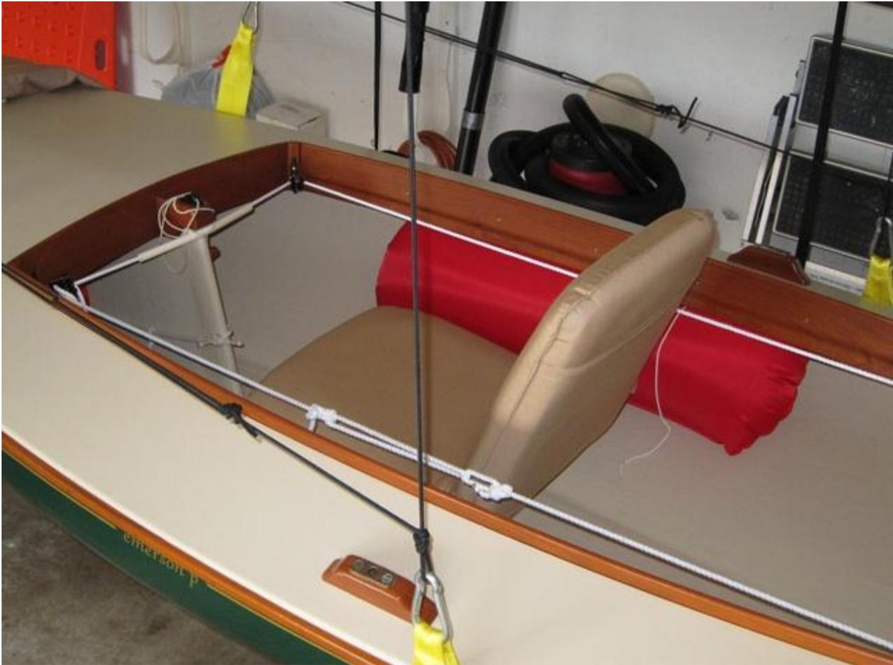
Here's a couple of edited pix. The yellow line is the main sheet. It will go forward from the block on the rudder to a port side block or fairlead hanging from the cross bar for the floats. From there, it will go forward to the top pulley of the double block in the forward port cockpit corner. From there, it will lead back to hand.
