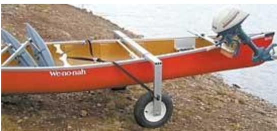
The wheels plug into the universal receiver bar, just like the floats. The only difference is they plug into both channels of the bar, instead of one like the floats do. Fore and aft swing of the wheel legs is controlled by nylon web straps across top of the boat. The Melonseed's fore and aft cockpit coamings should be great guides for these.
