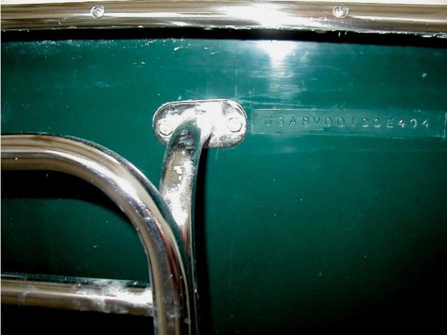
I drilled the hole next to the HIN first, and put a bolt through it. Then I leveled the tops of the two top brackets, and drilled the outer left hole. I put a bolt in it. Then, I drilled the rest of the holes using the brackets as drill guides. Measure and level a bunch of times, drill each hole only once!
