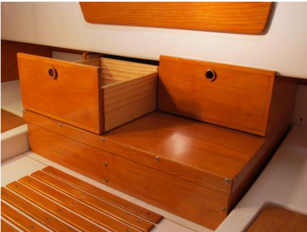
The step removed showing large storage area back to bulkhead.
