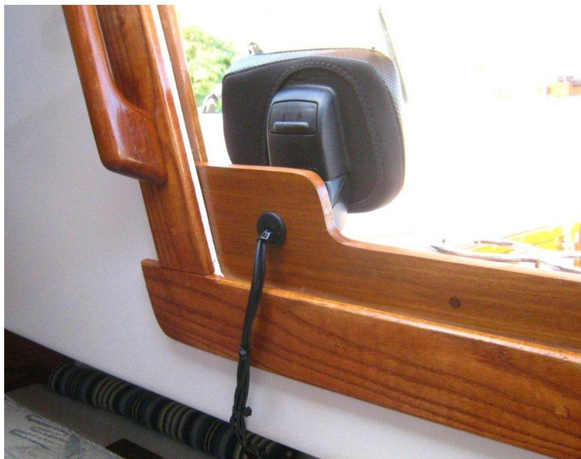
With the wiring (GPS, tranducer, and power) coming through the oak-veneered plywood that supports the bridgedeck, like this:
