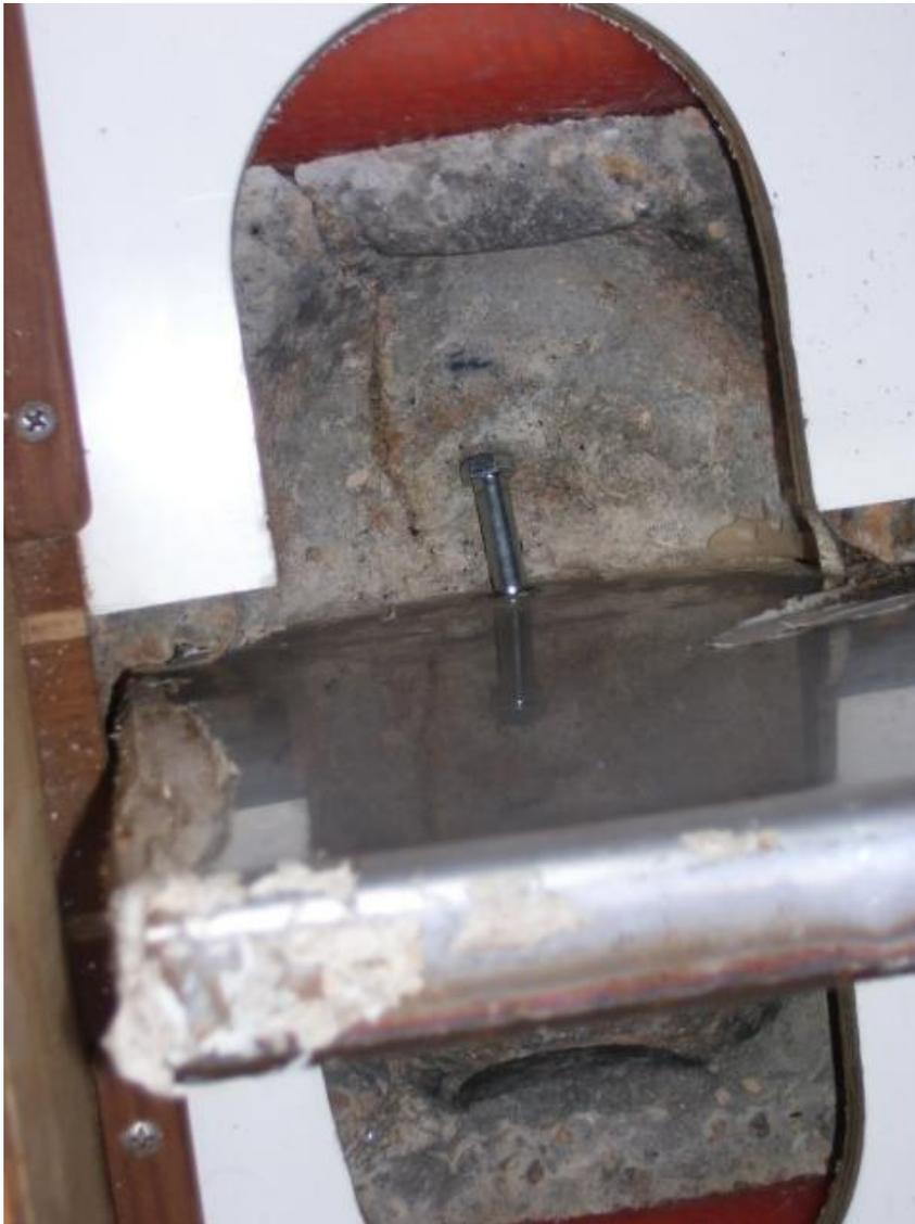
If the above doesn't stop the water, you've got a little project. I've included a photo to show you where I found a major leak in the centerboard pennant standpipe. That's the line that comes up through the floor of the cockpit through a pipe that you raise the centerboard with. You have to remove the teak block and make sure the hole is sealed.
